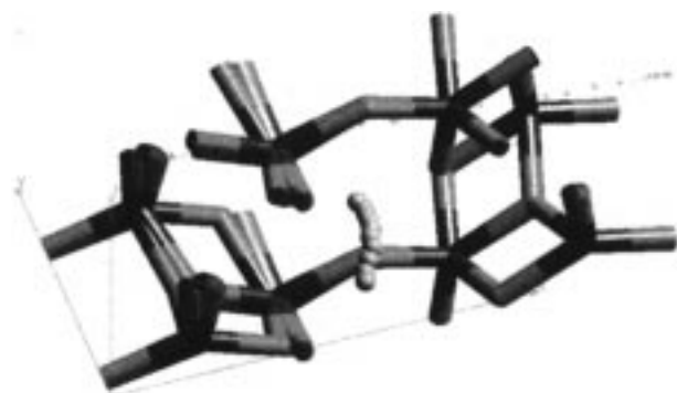
Figure 17. Lithium migration path through V_2O_5 for profile 1. Only the first half of the path is shown (from b = 0.0 to b = 0.5 ).
